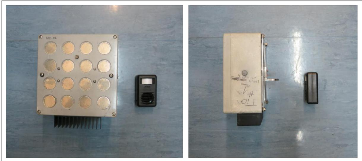
**Figure A9.4** – Comparison of Deaton (left in each picture) deterrent with CR deterrent (right in each picture). Shows front image (left) and profile image (right). Images: Matt Zeale
